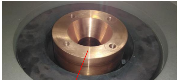
Massive non-cooled copper mould
